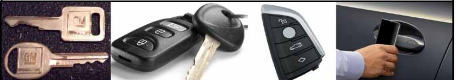
In 1998 the key fob made its debut. Remote entry key fobs locked and unlocked doors from several feet away by emitting a coded signal from it to a receiver in a car. Key fobs could also open trunks, sliding doors and start car engines. (Fob comes from the German word “fuppe” which means pocket.)
